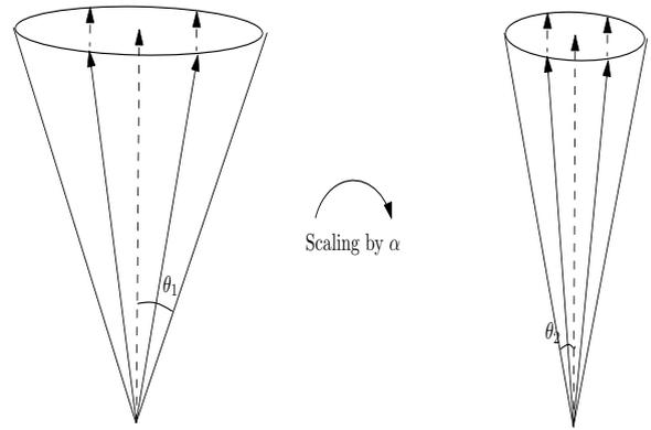
Fig. 5. Illustration of the scaling map (by an  $\alpha < 1$ ). A five element subset of the spherical cap shown on the left side is scaled to generate the set on the right side. In this operation, the following relationship holds true:  $\sin(\theta_2) = \alpha \sin(\theta_1)$ .
