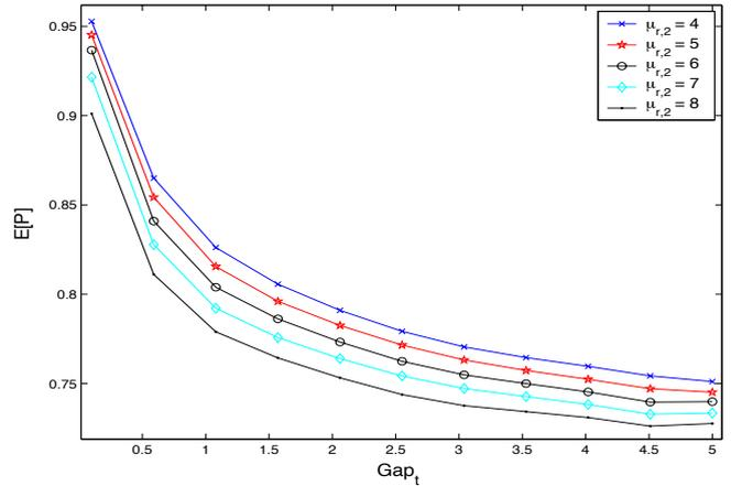
Fig. 2. Impact of  $\text{Gap}_t$  on  $E[P] = E[|\mathbf{u}_{\text{stat}}^H \mathbf{v}_1|^2]$  for a family of  $2 \times 2$  channels with a separable model and different values of  $\mu_{r,2}$ .
