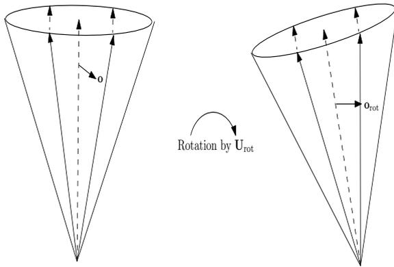
Fig. 3. Illustration of rotation of a five element subset of a spherical cap with center at  $\mathbf{o}$  by  $\mathbf{U}_{\text{rot}}$  to generate a corresponding subset of a spherical cap with center at  $\mathbf{o}_{\text{rot}}$ .
