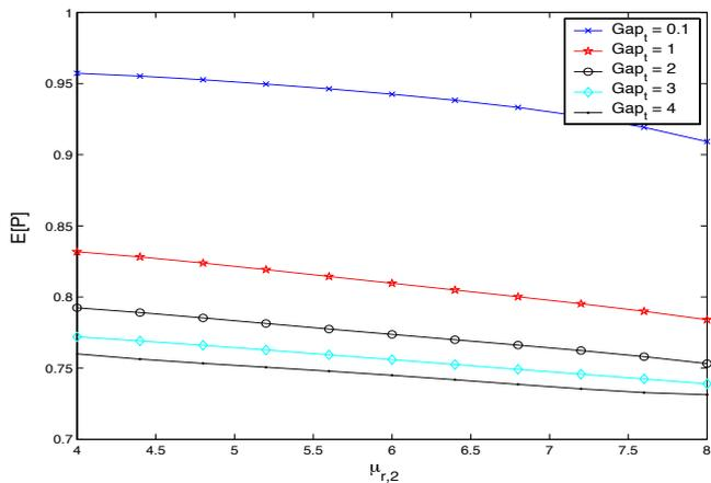
Fig. 1. Impact of  $\mu_{r,2}$  on  $E[P] = E[|\mathbf{u}_{\text{stat}}^H \mathbf{v}_1|^2]$  for a family of  $2 \times 2$  channels with a separable model and different values of  $\text{Gap}_t$ .
