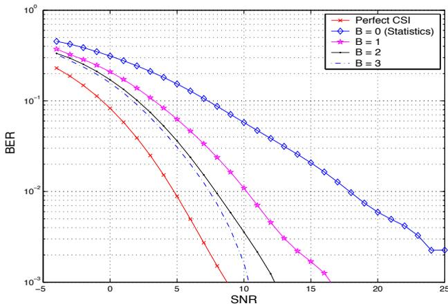
Fig. 7. Feedback performance in a  $1 \times 4$  channel generated with the separable model with transmit eigenvalues 1.38, 1.37, 0.99 and 0.26 resulting in  $\mu_r, 2 = 16$  and  $\text{Gap}_t \approx 10^4$ .
