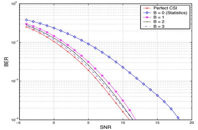
Fig. 6. Feedback performance in a  $2 \times 2$  channel generated with the separable model with  $\mu_{r,2} \approx 7.05$  and  $\text{Gap}_t \approx 148$ . The figure shows that even with as low as 1-bit feedback, substantial gains can be achieved with our codebook designs in extremely correlated scenarios.
