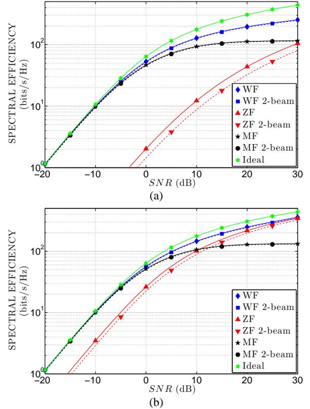
Fig. 3: (a) Capacity of three different B-MIMO precoders for downlink communication from an AP ( $n = 81$ ) to  $K = 40$  randomly distributed single-antenna MSs. (b) With minimum separation  $\Delta\theta_{min} = \frac{\Delta\theta_o}{4}$ .
