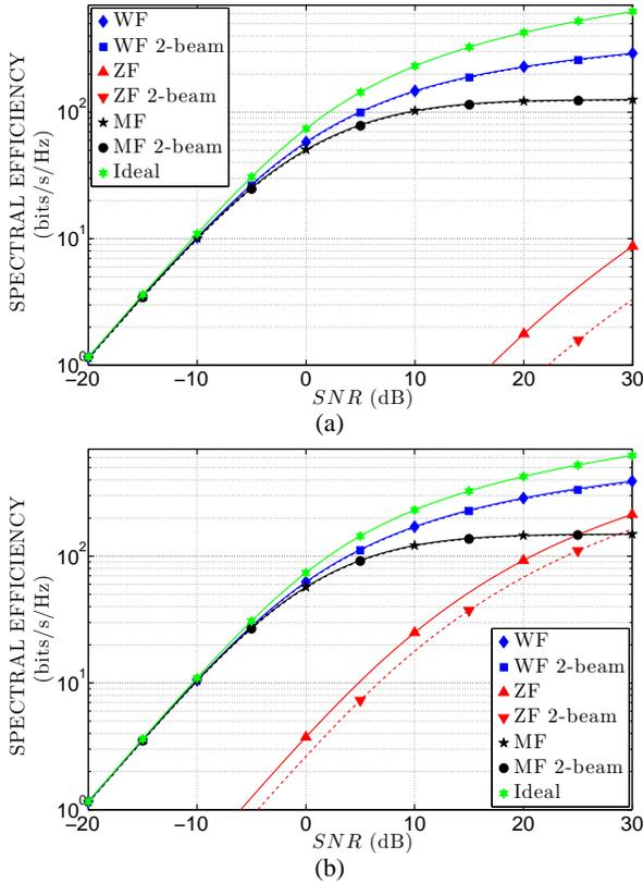
Fig. 4: (a) Capacity of three different B-MIMO precoders for downlink communication from an AP ( $n = 81$ ) to  $K = 60$  randomly distributed single-antenna MSs. (b) With minimum separation  $\Delta\theta_{min} = \frac{\Delta\theta_o}{4}$ .
