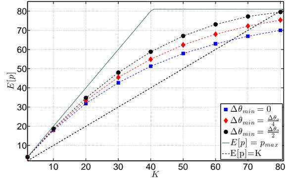
Fig. 5:  $E[p]$  (average number of selected beams) using the 2-beam sparsity mask when  $n = 81$ .
