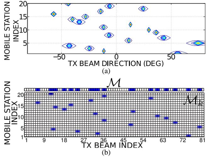
Fig. 2: (a) Contour plot of  $|\mathbf{H}_b^H|^2$  for a ULA with  $n = 81$ , representing the *beamspace channel vectors* (rows) for 20 MSs randomly distributed between  $\pm 90^\circ$  (b) Illustration of beamspace channel sparsity masks  $\mathcal{M}_k$  and  $\mathcal{M}$  for the  $\mathbf{H}_b$  in (a).
