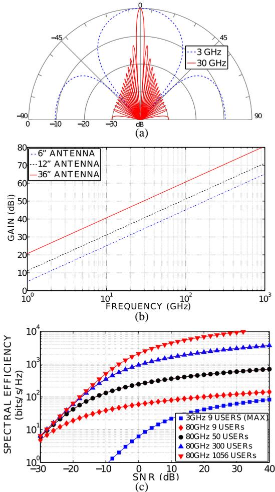
Fig. 1: (a) Antenna beampatterns for a 6" antenna at 3GHz vs. 30GHz. (b) Antenna gain vs. frequency. (c) Potential multiuser spectral efficiency gains due to spatial multiplexing at 80GHz vs. 3GHz with a 6" × 6" antenna.
