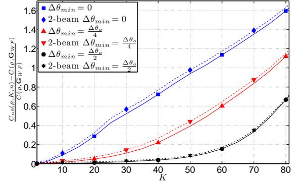
Fig. 6: Normalized capacity gap between the idealized upper bound and the WF precoder at an SNR of 30 dB
