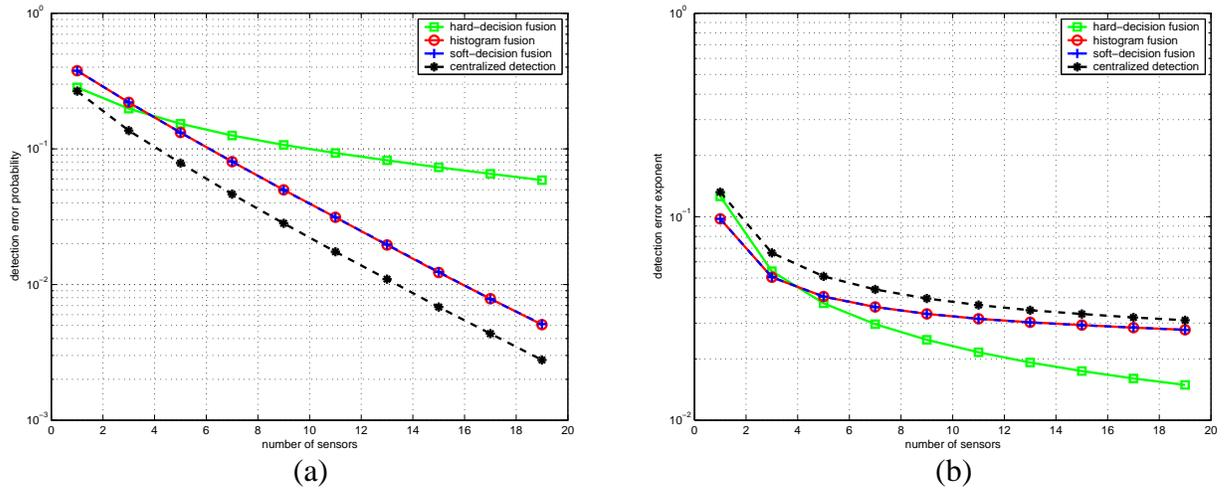
Figure 3: The performance of various detectors for the MAC under the IPC;  $P_{ind} = 5\text{dB}$ . (a) DEP as a function of the number of sensors ( $k$ ). (b) Error exponent of DEP as a function of  $k$ .
