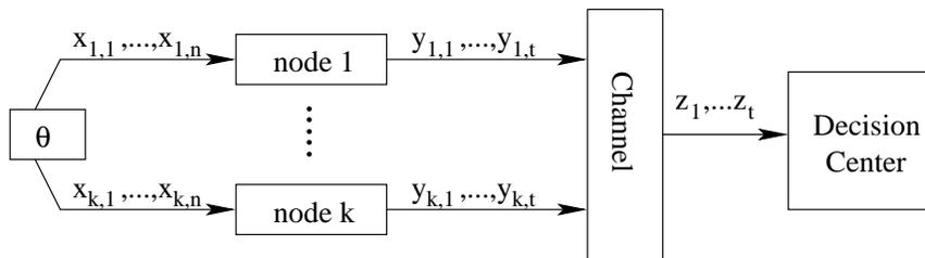
Figure 1: Architecture for decentralized detection using  $k$  spatially distributed sensor nodes. The sequence  $\mathbf{x}_i = (x_{i,1}, \dots, x_{i,n})$  denotes the observation data at node  $i$  ( $1 \leq i \leq k$ ). The observations are generated according to a distribution  $Q_\theta$ ,  $\theta \in \{\theta_0, \theta_1\}$ .
