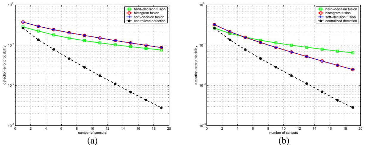
Figure 4: DEP as a function of  $k$  for the MAC under the TPC. (a)  $P_{tot} = 5\text{dB}$ . (b)  $P_{tot} = 10\text{dB}$
