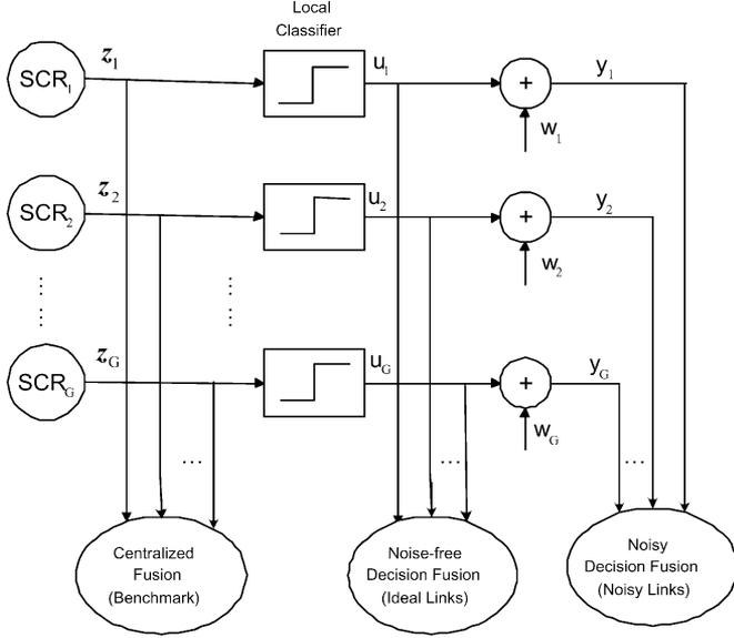
Fig. 1. Generic architecture for multitarget classification. All classifiers operate on  $G$  i.i.d. feature vectors  $\{z_1, \dots, z_G\}$  collected in distinct SCRs. Local hard decisions from the SCRs are communicated via ideal or noisy links to a manager node that makes the final decision.
