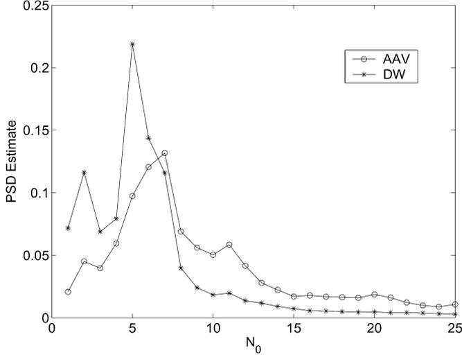
Fig. 3. Covariance matrix eigenvalues (PSD estimates) of acoustic measurements for the two target vehicles.
