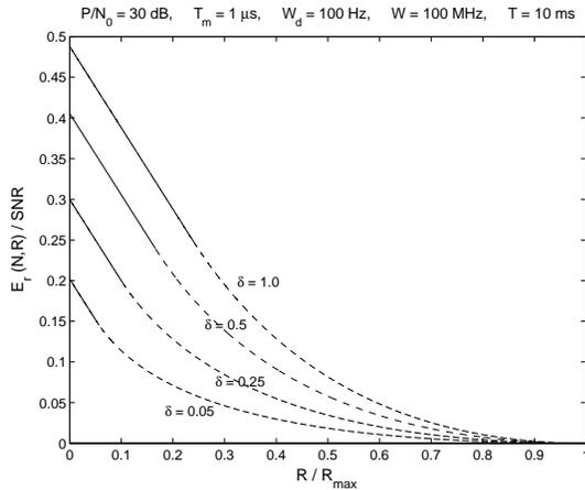
Fig. 2.  $E_r(N, R)/\text{SNR}$  vs. normalized transmission rate with perfect CSIR. Effect of varying  $\delta$ . Solid line denotes the linear portion ( $\rho^* = 1$ ) and the dashed line is the region where  $0 < \rho^* < 1$ .  $R_{cr}$  defines the boundary between the two regions.
