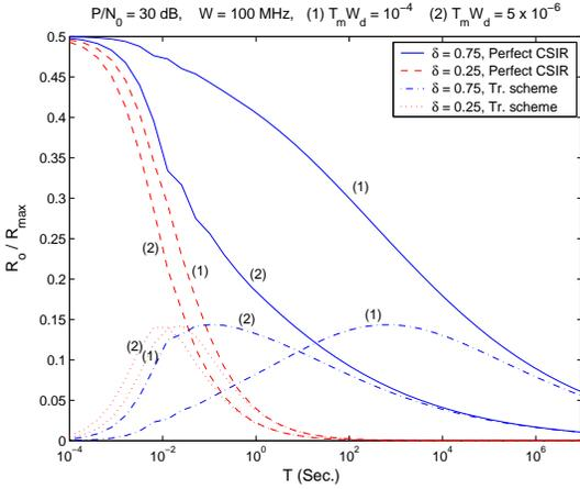
Fig. 6. Cut-off rate vs.  $T$  for perfect CSIR and training-based communication schemes
