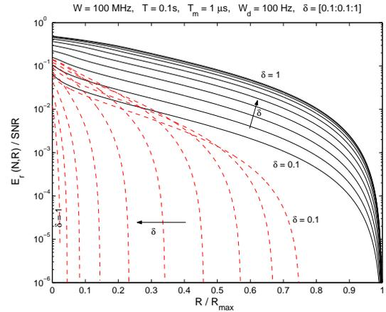
Fig. 4.  $E_r^{tr}(N, R)$  for a family of sparse channels; Solid lines denote the perfect CSIR case while dashed lines denote the training-based scheme
