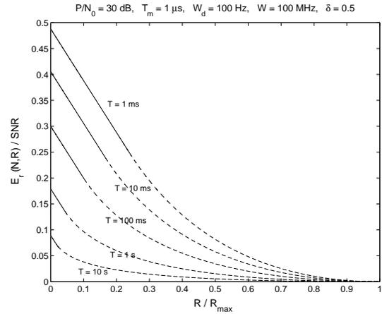
Fig. 3.  $E_r(N, R)/\text{SNR}$  vs. normalized transmission rate with perfect CSIR illustrating the effect of increasing signaling duration
