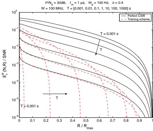
Fig. 5. Effect of changing signaling duration  $T$  on  $E_r^{tr}(N, R)$  for a sparse channel with  $\delta = 0.4$
