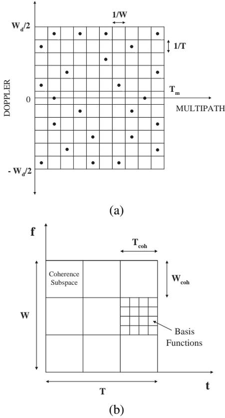
Fig. 1. (a) Delay-doppler sampling commensurate with signaling duration and bandwidth. (b) Time-frequency coherence subspaces in short-time Fourier signaling.
