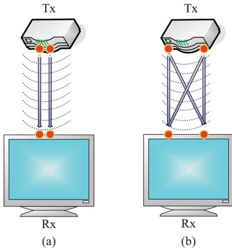
Fig. 1. Schematic illustration of (a) conventional and (b) optimized MIMO systems in LoS. The former configuration offers minimum multiplexing gains due to the high correlation between the LoS responses whereas the latter delivers orthogonal LoS subchannels.
